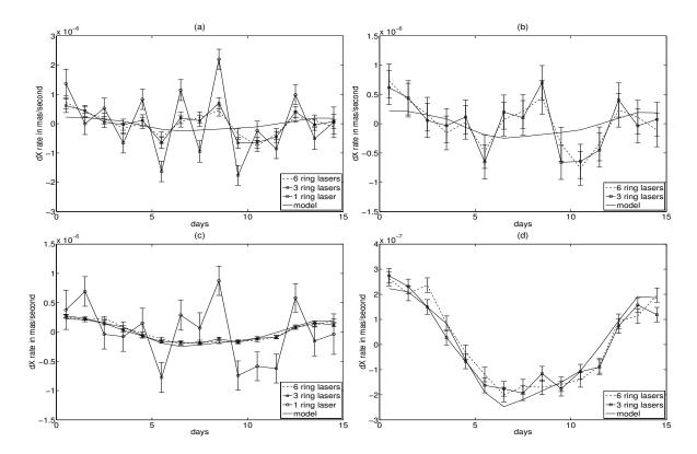
**Fig. 21.** Nutation rates from VLBI and RLG combined solution. Plots (a) and (b) show results for an assumed RLG accuracy level of 10-9 and (c) and (d) for 10-10. Note the different scales on vertical axes. From (Tercjak et al., 2015)
