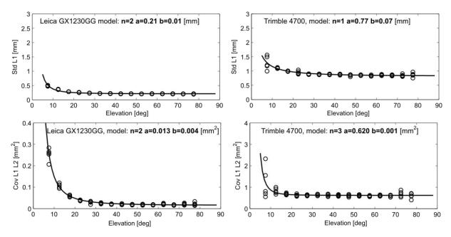
**Fig. 11.** Empirical stochastic models for L1 standard deviation (top) and L1/L2 covariance (bottom) for two tested receivers: Leica GX1230GG (left) and Trimble 4700 (right)
