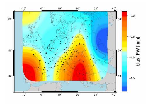
**Fig. 20.** IPW difference (GNSS EUR tropospheric combination - COSMO-LM\_14; annual average) map for 2011, meteo from COSMO model GNSS networks provide us with vertically integrated humidity information (precipitable water) which can feed COSMO model (nudge water vapour content in right direction) in network much denser then radiosoundings
