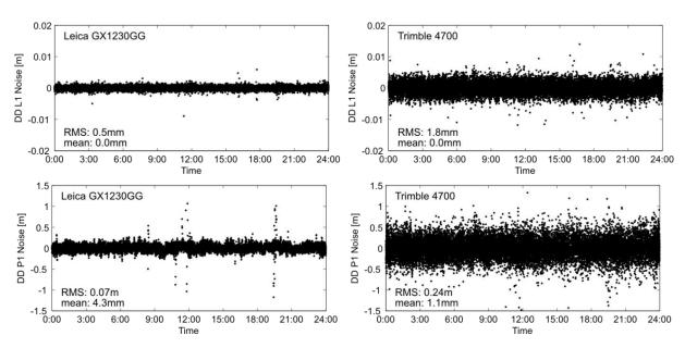
**Fig. 10.** GPS signal noise of DD phase for L1 (top) and code for P1 (bottom) observations for two tested receivers: Leica GX1230GG (left) and Trimble 4700 (right)
