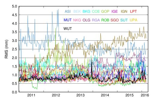
**Fig. 6.** RMS of position residuals after Helmert transformation between each EPN AC weekly solution and the combined weekly solution. Thicker black line shows RMS values for WUT analysis centre
