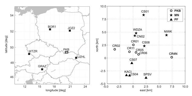
Fig. 22. Map of datum definition sites (left) and points of PKB geodynamic test field (right)
