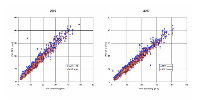
**Fig. 13.** Legionowo radiosounding IPW vs. GPS JOZE in 2002 and 2003: dark points - original EPN combination, bright points – WUT LAC reprocessing
