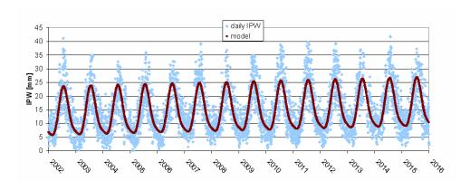
**Fig. 17.** IPW for JOZE (Józefosław) and linear model with 2 oscillations (annual and 1/2-year) applied to 2002-2015 period, IGS tropospheric solution, IPW trend in this case is evident: 0.25 mm/year
